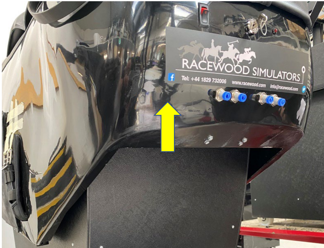
Image 1: Damper located inside fibreglass bodyshell at the front of the simulator.
