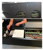
While someone pushes the push scale to **2.5Kg** on the required sensor, using a small screwdriver adjust the screw on the small blue terminal that is marked as the correct one for that sensor. (eg, L1, L2)
